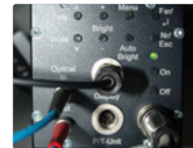
Rear of camera module with fibers connections and battery power supply cable
