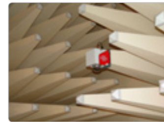
Camera fixed on pyramid absorbers
