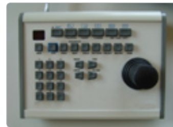
Controller for CCTV and Intercom
