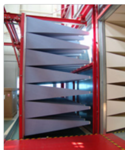
Sliding door with pyramid absorbers
