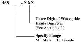
For Example: **Mi-Wave'** model number 365 F-495 is a circular load for a frequency range of 34.8 to 48.0 GHz with an inside waveguide diameter of 0.500" inches.
