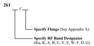
For Example: Model number 261 W/387 is a standard gain horn operating in W-band with a 387 type flange.
