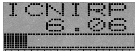
SPECTRAN® displays exposure limits both as percentage as well as a bargraph display.
